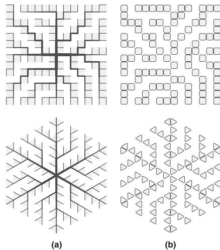
FIG. 3. Networks that are easy to repair after one break. The original networks (a) and the overlapping dormant loops (b).
