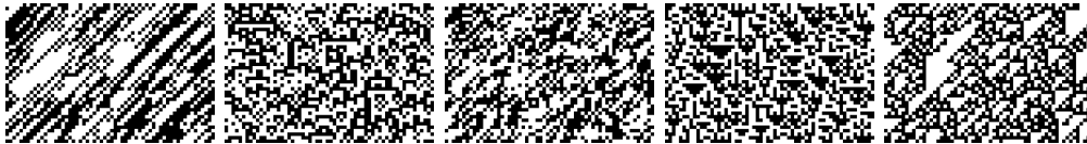
FIG. 3: Simulation-generated pictures for some representative samples of random probabilistic cellular automata. In all of these automata the probability that a cell is coloured is \frac{1}{2} . The rules, from left to right, from a_7 to a_0 are given at the end of this manuscript [30].
