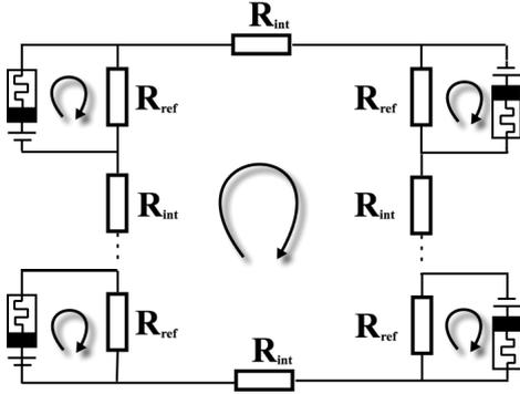
FIG. 1: More general case with  $n$  memristors arranged on a loop. Since the circuit is planar, all the loops can be chosen with the same orientation.
