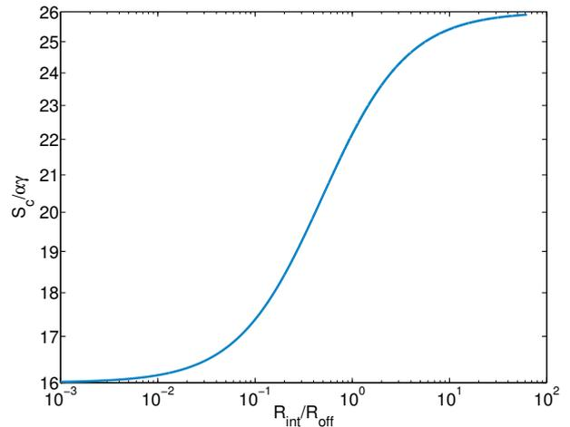
FIG. 2: Critical line of eqn. (11) of the non-equilibrium dynamics starting from switched off memristors,  $w_i(0) = 1$ . Parameters of the model:  $R_{ref} = 1000$ ,  $R_{on} = 100$ ,  $R_{off} = 1600$ , and  $\alpha = \gamma = 1$ .
