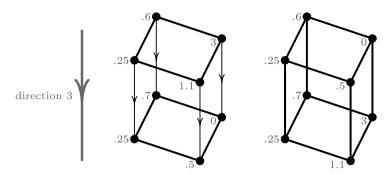
**Fig. 1.** A  $C_{(3),\emptyset}$ -compression in  $Q_3$ . (In each edge marked by an arrow, the coordinates of the two vertices are swapped if the coordinate at the starting point is larger than the coordinate at the end point.)
