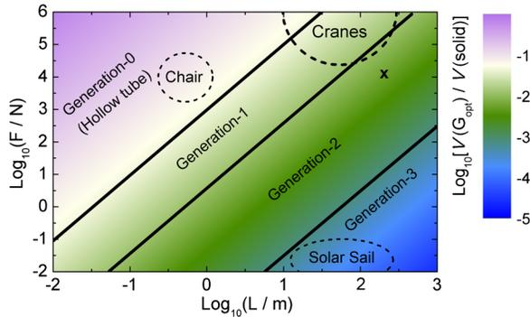
FIG. 4 (color online). The material saving for a given  $F$  and  $L$  over a solid beam assuming material properties close to those of steel. Also depicting the progression of optimality from simple structures (chair legs) to structures with many levels of hierarchy. Also shown is the point  $F = 10$  kN,  $L = 200$  m ( $\times$ ) and the regions appropriate for construction of a solar sail compression beam and the boom of a crane [20].
