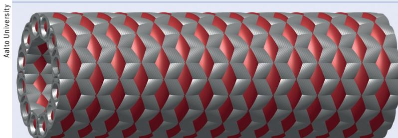
This diagram shows a first-generation pressure-bearing structure. In higher-generation structures, each of the cylindrical sub-structures would be replaced by a scaled version of the whole structure. The design shows remarkable efficiency under gentle pressure loading, and the structure on the largest length scale does not have to be a cylinder – any convex shape constructed with this same substructured material will display the same efficiency gains.
