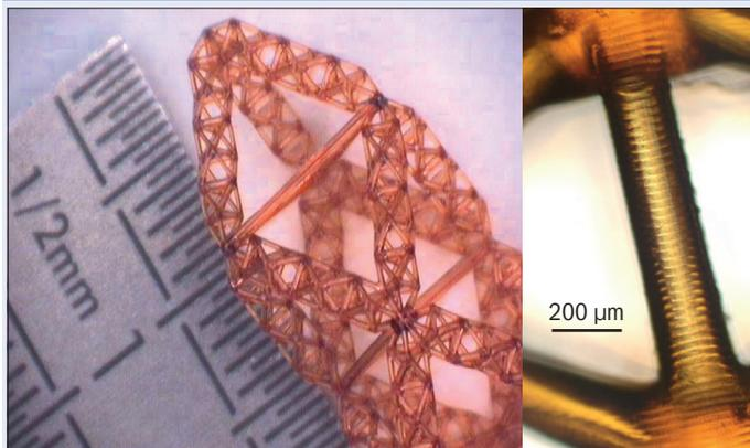
This frame was constructed using a 3D printing technique known as stereolithography. In this technique a photopolymer is exposed to light only in regions where solid material is required. The inset shows the layered nature of the material, which is a consequence of the layer-by-layer printing process.
